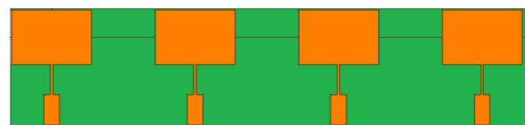
Fig.4: Schematic of setup of FECMAA for mutual coupling measurement.
