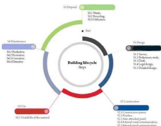
Figure 1: The life cycle of the building and its stages. Source: prepared by the author with data from ISO 14044 (2009)
