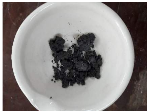
Fig.1: Extracted silicon from sand after leaching out
