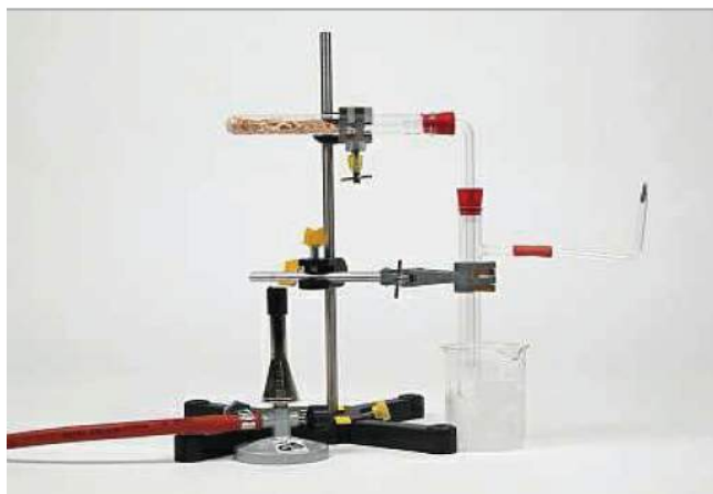
Figure 1: Kiln for Extracting Wood Vinegar
