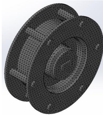
Fig. 9: Mechanical Drawing of the ISCT200-US Thruster With the Subdivision of the Solid Into Finite Elements
