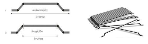
Figure 1: Dramix type of Steel Fiber
