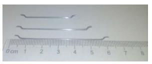
Figure 8: Hooked End Steel Fiber Used
