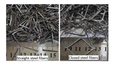
*Figure 11:* Steel Fiber Used that Cut Manually
