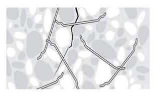
Figure 12: Mechanical Interlock of SFRC
