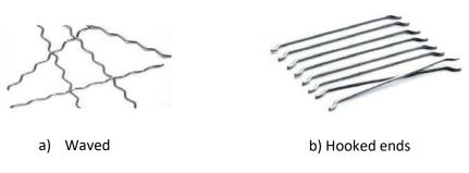
*Figure 4:* Types of steel fiber used
