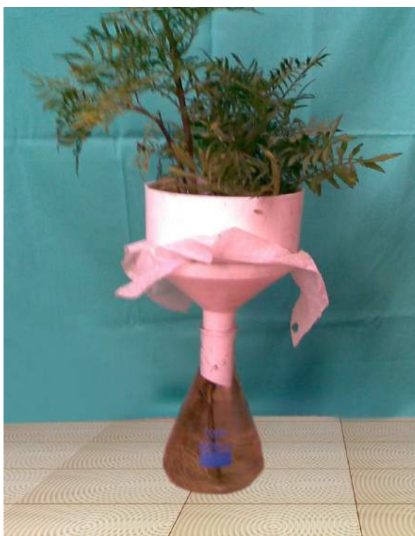
Fig.1: Marigold plant grown in root exudates trapping system
