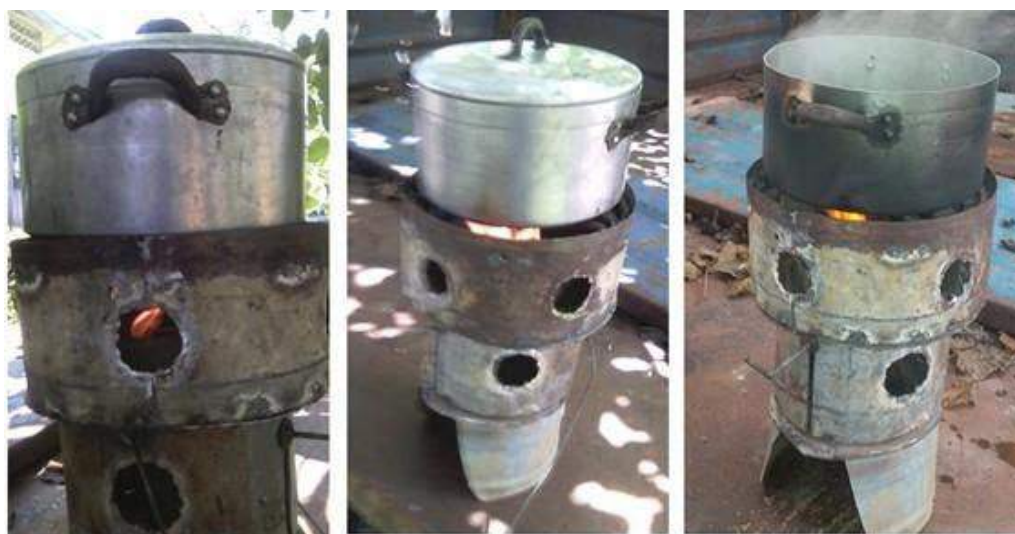
Figure 3: Water boiling and cooking test setups
