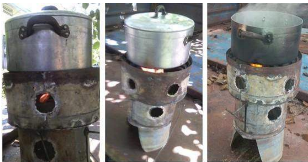
Figure 3: Water boiling and cooking test setups
