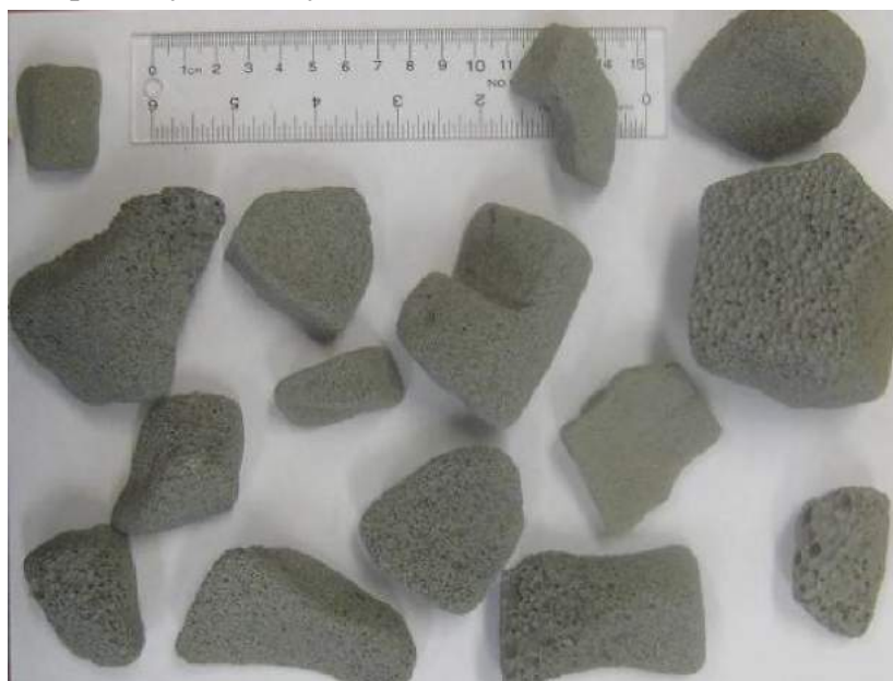
Figure 3: Chunks of glass foam for insulation under roads
