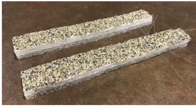
Figure 4: Long and narrow tiles with mineral grains adhered on one side
