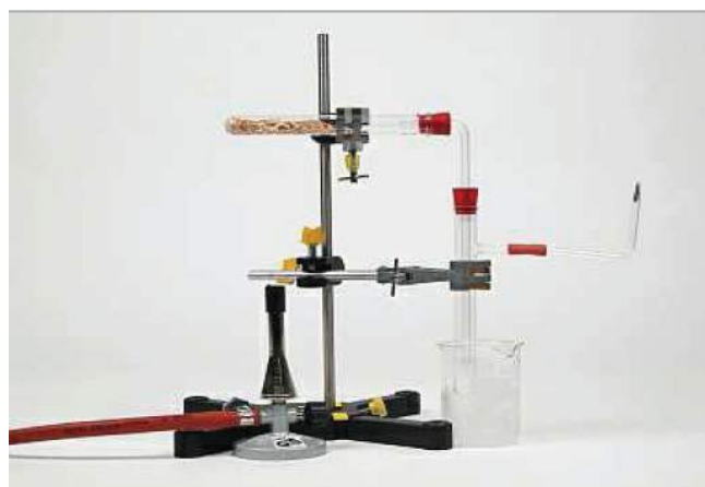
Figure 1: Kiln for Extracting Wood Vinegar
