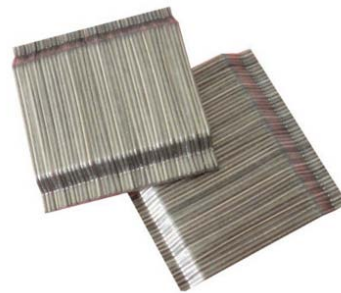
Figure 2: Steel Fiber Hooked-End Type Glued in Bundles
