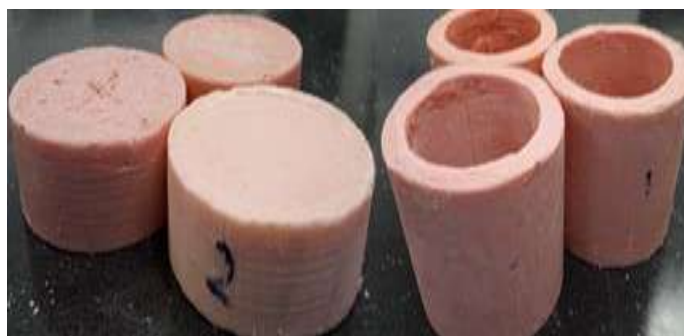
Figure 3: SEQ Figure:_3. \* ARABIC 1 Constructed Soft Scale (a) Solid Shaped, (b) Hollow Shape Samples [23]
