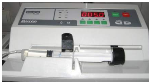
Fig. 3: Portable metering device for cisplatin introduction
