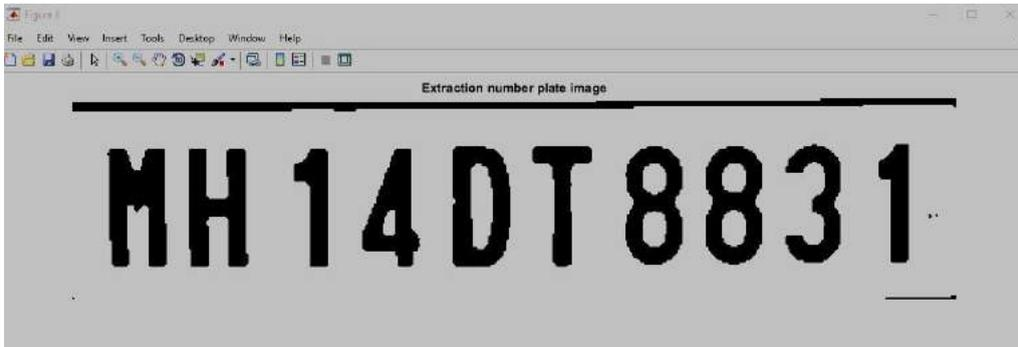
Figure 8: Extraction of number plate.
