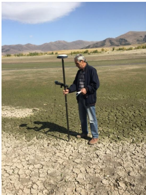
Fig. 2: Coordinate measurement of the deposit surface by the rover
