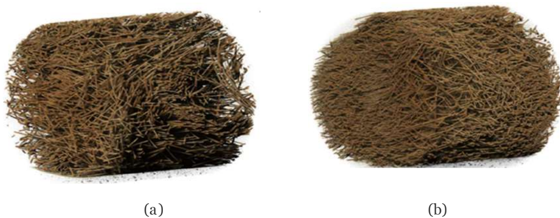
Figure 6: Synchrotron Scans Rendered in ORS Dragonfly: (a) Quartz Felt; (b) High-Density Quartz Felt
