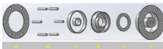
Fig. 5: Exploded View of the Mechanical Drawing of the ISCT200-US Thruster. From Left to Right: (a) Base Piece, (b) 6 Tubes for Heat Transmission, (c) Representation of Permanent Magnets, (d) Ceramics, (e) Anode, and (f) Structure
