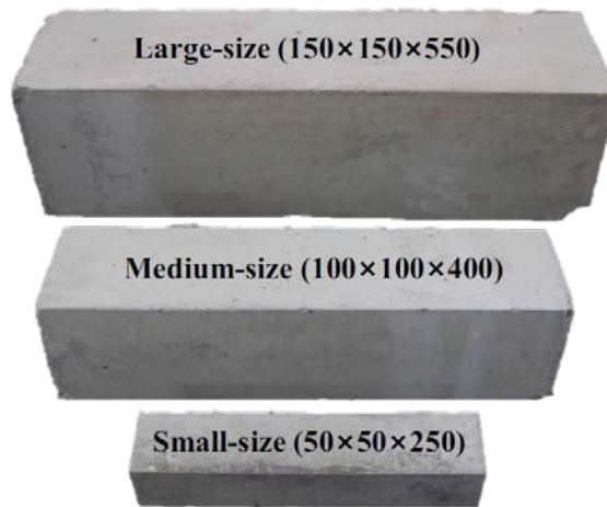
Figure 6: Geometry of Specimens Used (Units: Mm)
