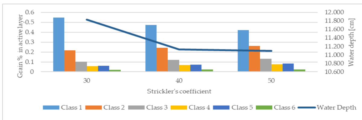
Figure 2: This Is a Plot of the Final Percentage of Grain Class in the Active Layer of the Riverbed and Corresponding Water Depth at Constant Shield's coefficient of 0.040 and Strickler's coefficients at 30, 40, and 50
