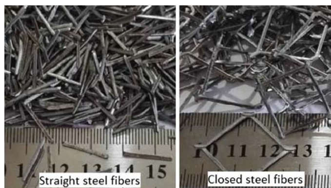
Figure 11: Steel Fiber Used that Cut Manually
