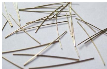
Figure 9: Straight Steel Fibers used
