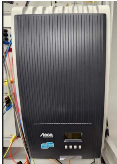
(b) PV inverter
