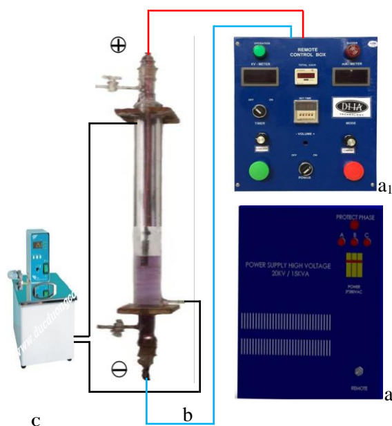
Figure 2: Model of DC high voltage equipment
