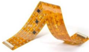
Figure 1: FPCB with installed EC – electronic unit
