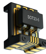
Figure 5: 3D-MID mechatronic unit
