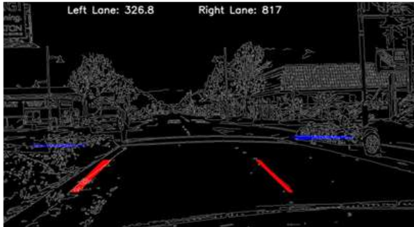
Fig. 6: Left and Right Lane Estimation with lane boundaries in Grayscale
