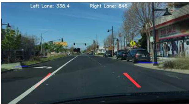
Fig. 6: Left and Right Lane Estimation with lane boundaries in Grayscale
