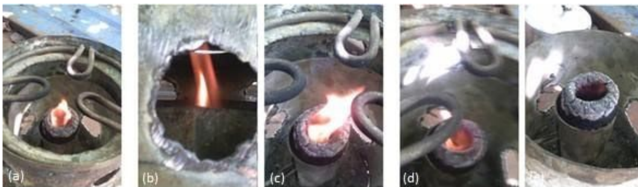
Figure 2: Flame propagation of briquette in stove combustion chamber
