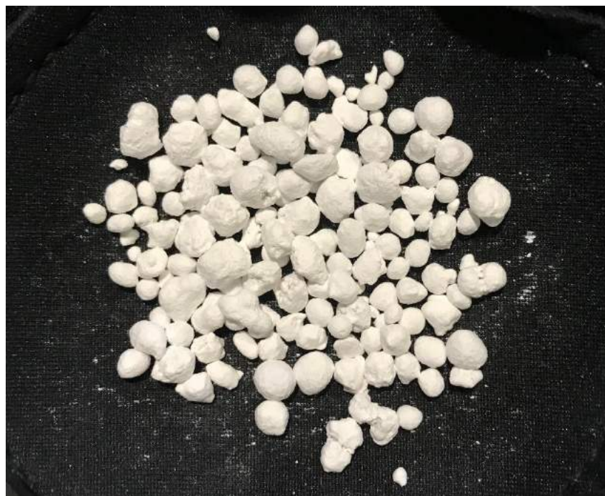
Figure 5: AGSCO (Wheeling Illinois) glass foam beads coated with adhered chalk dust
