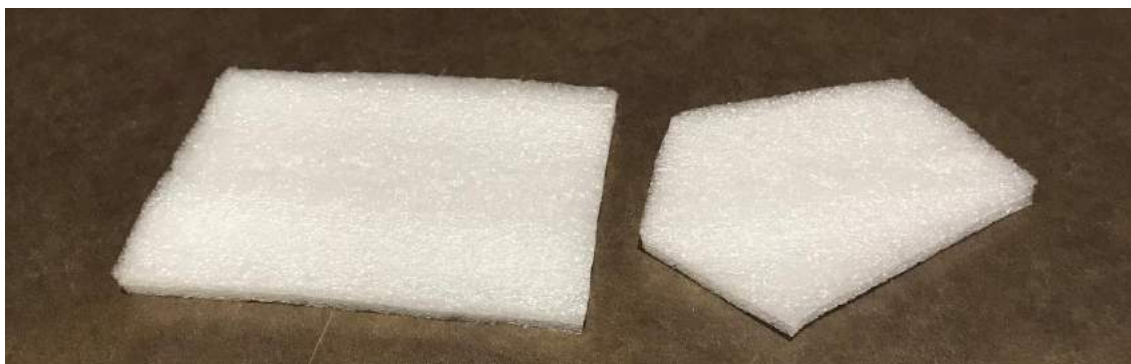
Figure 2: Models of glass foam tiles
