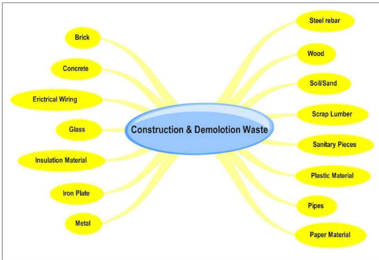
Figure - 4: Construction & Demolition Waste
