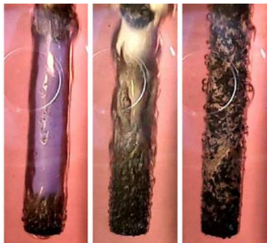
Fig. 8: Polymeric surface layer formation during quenching standard probe in oil [17, 18].
