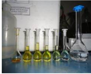
Figure SEQ Figura \* ARABIC 4: Standard \beta -carotene solutions and calibration ratio
