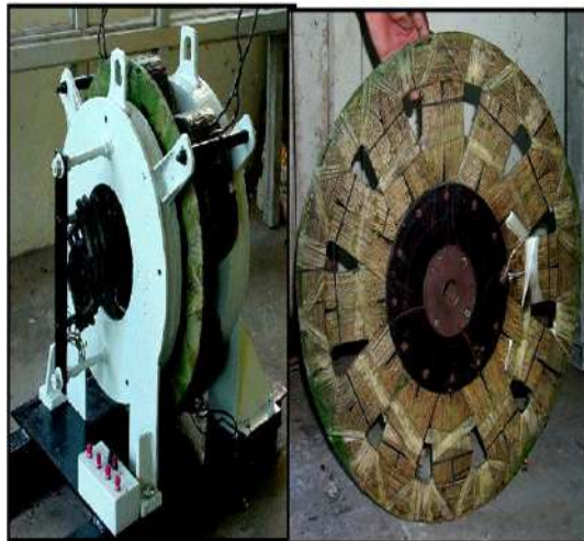
Fig. 6: Low Reversibility Electric Generator (2004), on the Right Its Rotor
