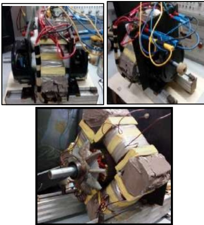
Fig. 8: Experiment to Study Electromagnetic Torque in a Hasselwander Generator. Above: Side and Diagonal View. Below: The Rotor - Stator Assembly in a Demonstration Photo of Physical Layout
